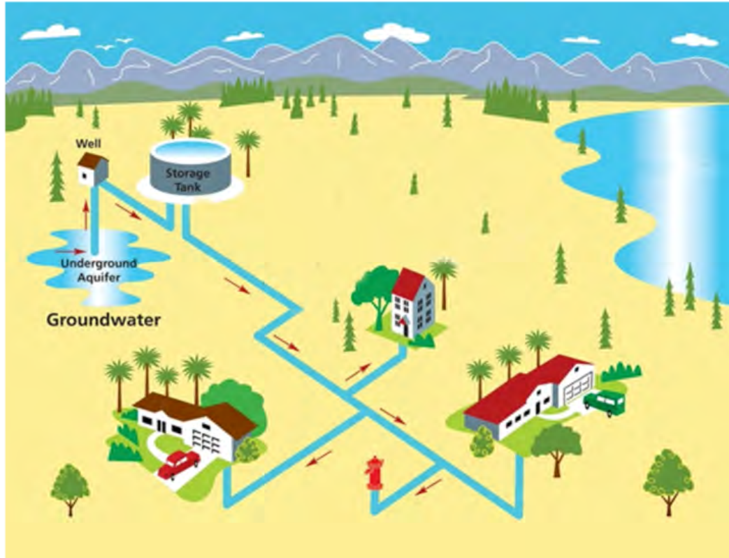
Figure 13. Conceptual schematic of a new CWS. Image courtesy of California Water Service.
