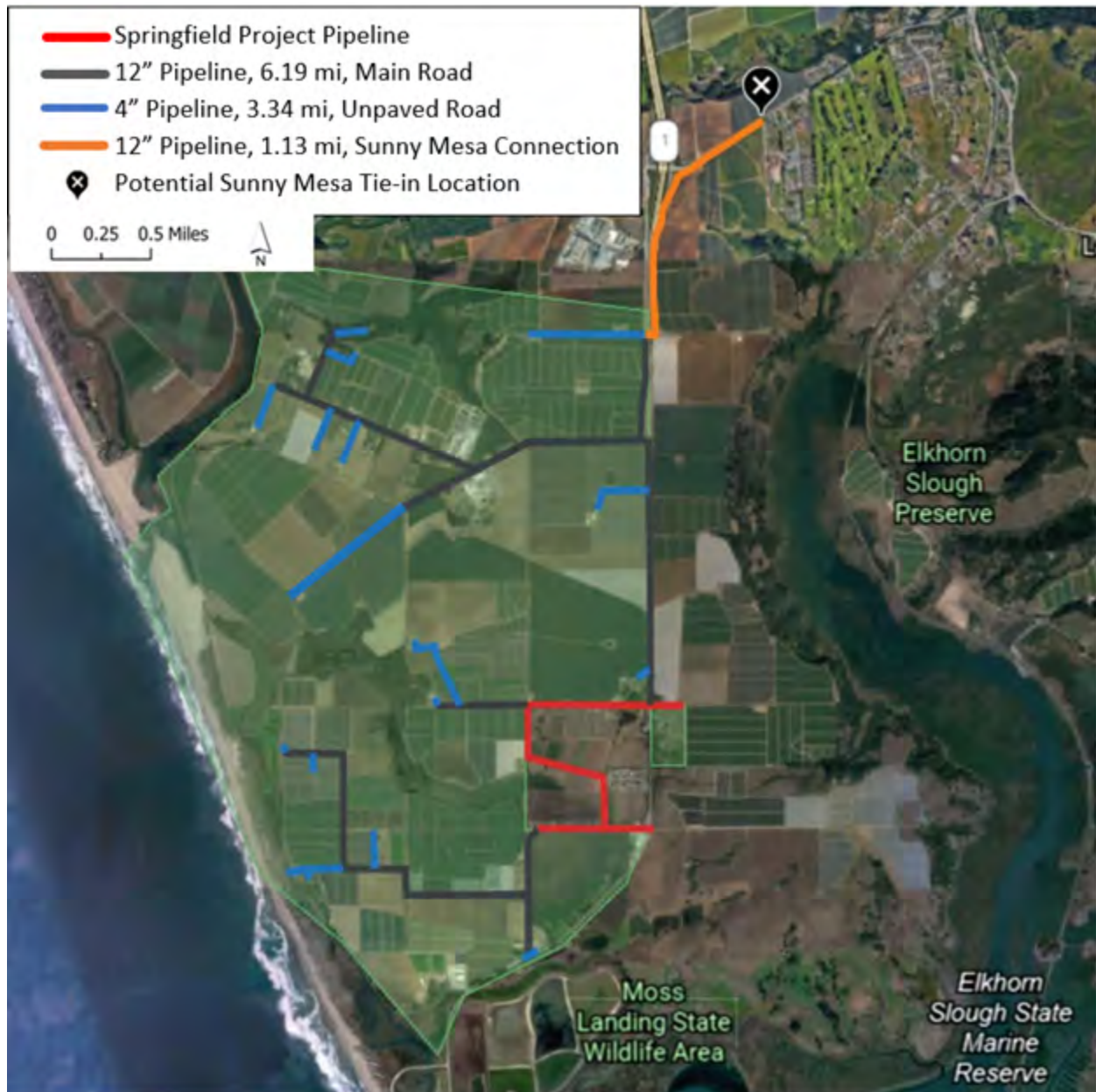
Figure 12. Conceptual map of Scenario B: Physical consolidation with the Springfield Project and Sunny Mesa and Pajaro Systems.*
